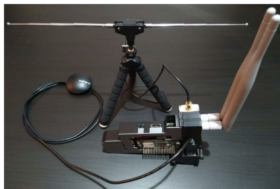
Figure 3: L.A.N.C.E.D. Mark I device mounted with GPS, GPRS, SDR and two NICs
